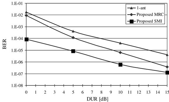
**Fig. 13** BER evaluation in radio environment II.
