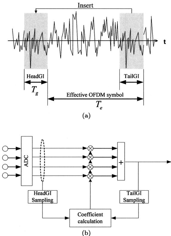
Fig. 1 (a) The periodic property of OFDM signal and (b) principal array antenna utilizing GI.
