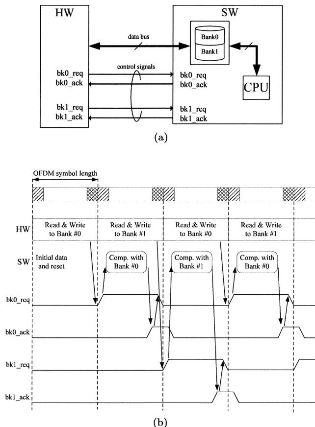
Fig. 5 (a) HW-SW interface and (b) timing diagram of array antenna.
