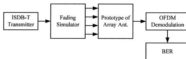
**Fig. 8** Block diagram of the experiment system.**Table 4** Multipath environment to verify the operation of the array antenna.
