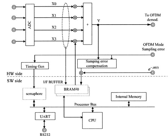
Fig. 4 Functional block diagram of joint HW-SW solution for array antenna.
