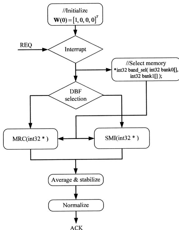
Fig. 6 Operation of CPU.
