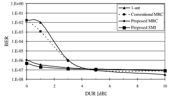
Fig. 11 BER evaluation in radio environment I with Delay=21 μs.
