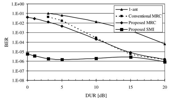
Fig. 12 BER evaluation in radio environment I with Delay=147 μs.
