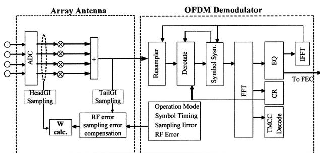
Fig. 2 Block diagram of OFDM reception.
