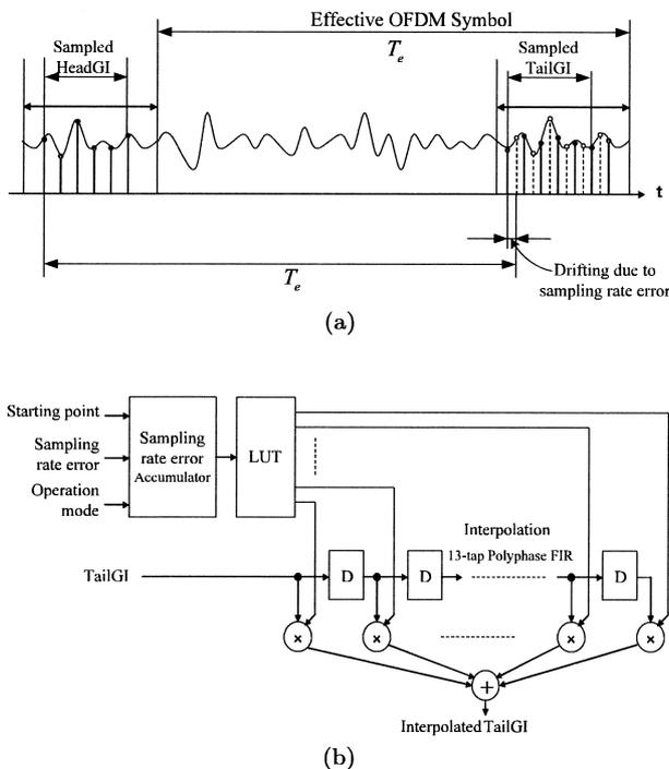
Fig. 3 (a) Impact of sampling rate error and (b) block diagram of the compensation of sampling rate error.
